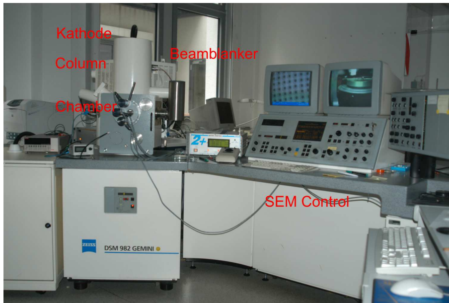
Figure 2: Low Voltage Scanning Electron Microscope Zeiss Gemini DSM 982 with beam blanking attachment
