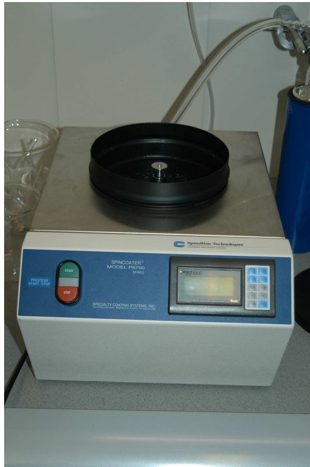
Figure 23: Spin-coater for preparation of thin resist layers
