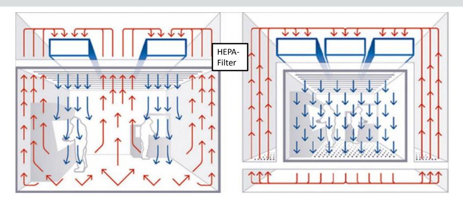
"dilution effect"- non-parallel /nonuniform flow streams and velocities. clean air entering the room and diluting the contaminated air.
