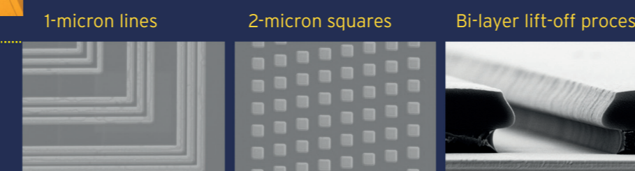
1-micron lines 2-micron squares Bi-layer lift-off process
